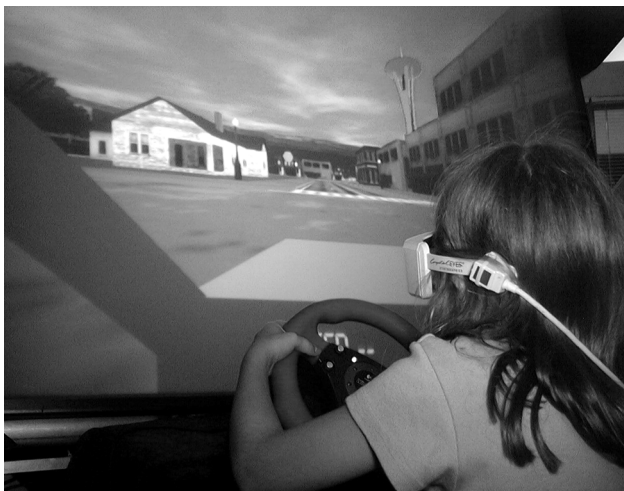
Figure 22 Steering a vehicle is one way in which the user can use a physical device to interface with the virtual world. (Copyright 2003, William Sherman.)
