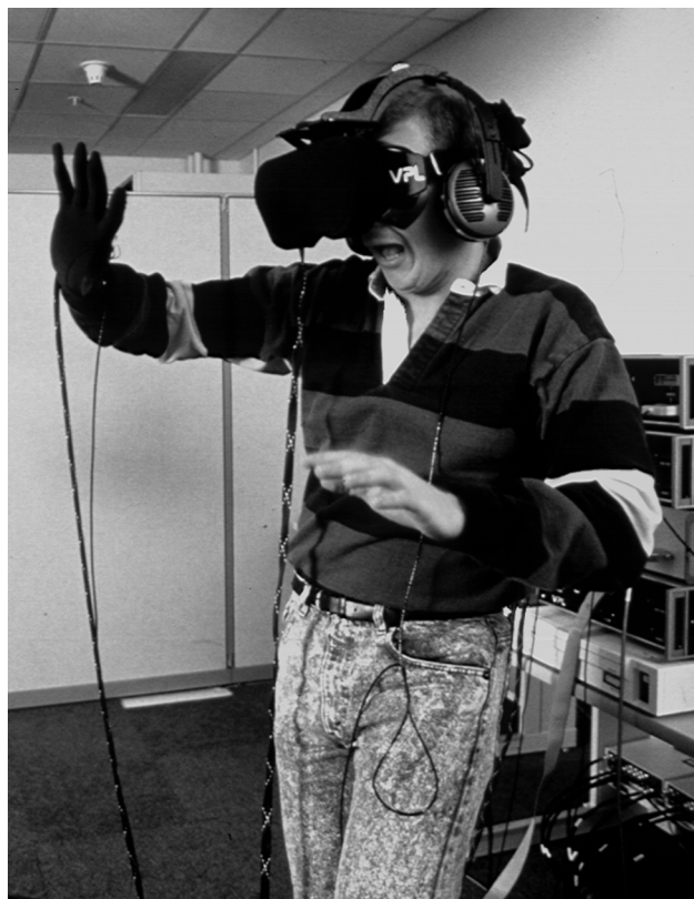
Figure 1 A virtual reality participant wearing a head-mounted display and a glove input device interacts with a virtual world. (Image courtesy NCSA.)
