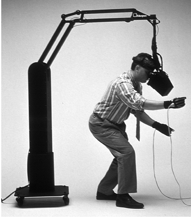
Figure 12 The BOOM head-based display mounts the screens on an arm that takes the weight from being applied to the user's head. (Image courtesy Fakespace Systems, Inc.)
