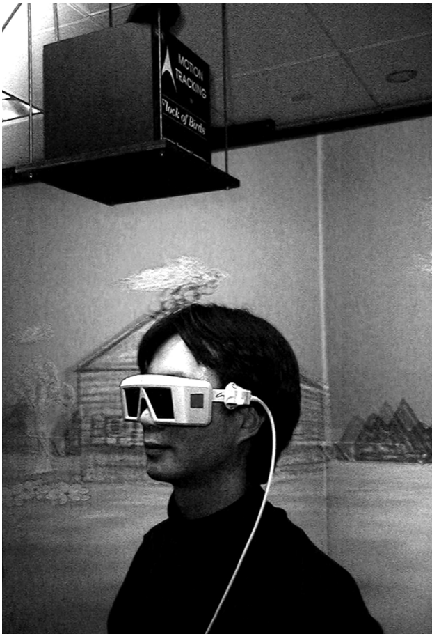
Figure 17 A low-level electromagnetic field is emitted by the large black box. The signal is sensed by a receiving antennae which allows the system to determine the location and orientation of the receiver. (Copyright 2003, William Sherman.)
