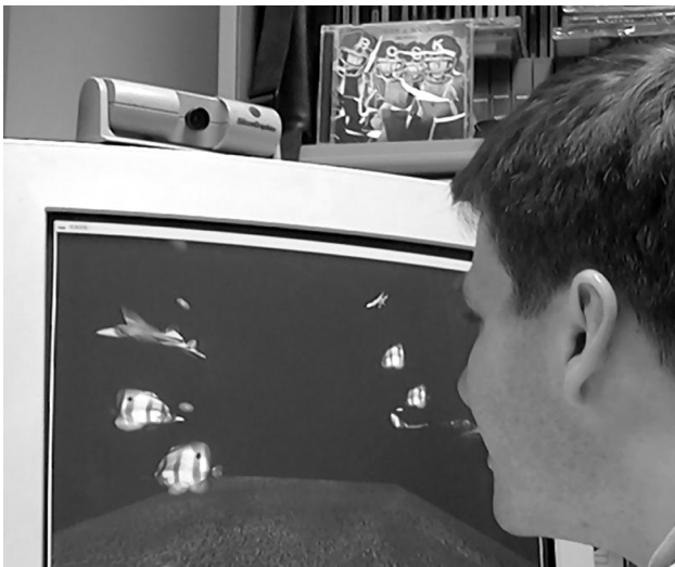
Figure 14 A computer monitor with a video camera can be a very simple VR display, referred to as “fishtank VR” due to the similarity with looking into an aquarium. (Copyright 2003, William Sherman.)
