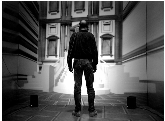
Figure 11 The stationary CAVE visual display and loudspeaker aural display are often used together. (Copyright 2003, William Sherman.)
