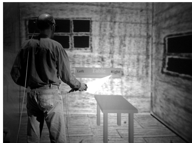
Figure 23 Interacting with a graphical (virtual) controller is an example of a virtual input interaction, such as moving this table using a virtual slider. (Copyright 2003, William Sherman.)
