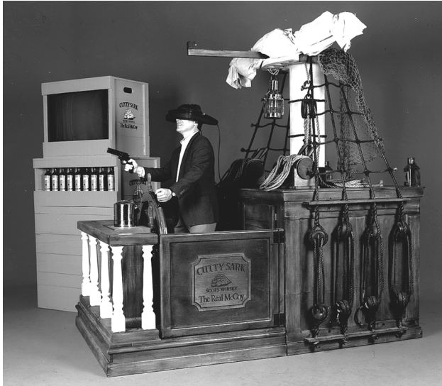
Figure 19 In this virtual reality system, a platform with a ship's wheel mounted on it provides the space where the participant takes their virtual voyage. (Image courtesy Randy Sprout.)
